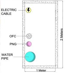
Representative section of Underground Utility duct
